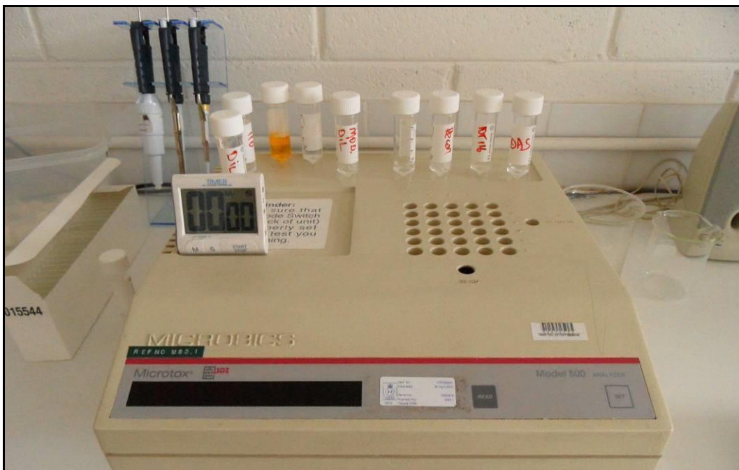
Plate 18 Temperature controlled photometer apparatus used to test for bioluminescence of Vibrio fischeri in the 30 min EC 50 test.
